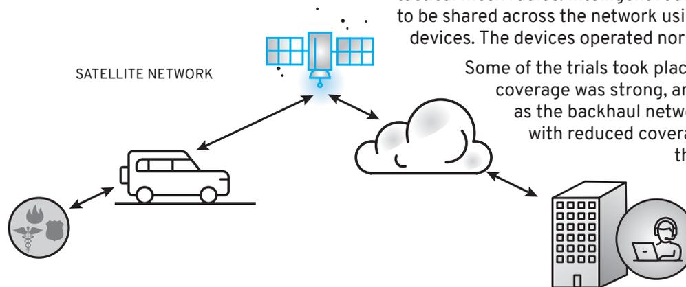
Some of the trials took place in areas where local cellular coverage was strong, and the hybrid solution selected that as the backhaul network. As the operation moved to areas with reduced coverage, the hybrid network switched the backhaul to the satellite network and operations continued with no notable outage to the end user. Using this hybrid network, agents were able to continue their standard operations well beyond the terrestrial coverage areas.
