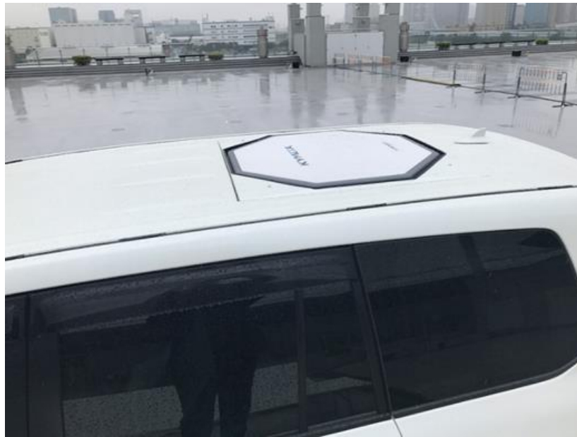
Figure 7. The 70 cm Ku-band antenna product mounted flush in the roof of a test vehicle
