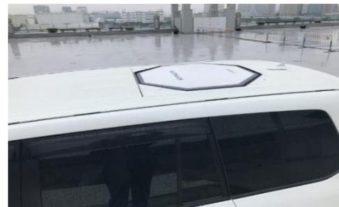
Fig. 8. The 70 cm integrated terminal installed in the roof of a Toyota Land Cruiser.
