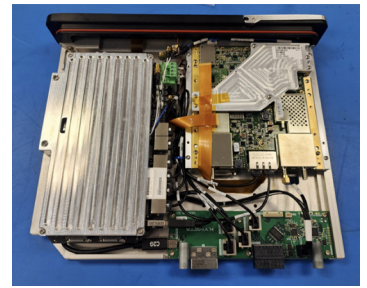
FIGURE 2 Field-removable Modular Modem Cartridge
